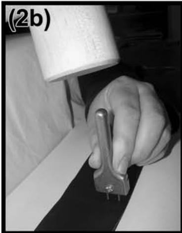
2b) An alternative awl is the dual-blade awl, it makes two slits at once.
